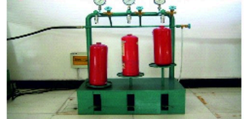
Hydro Testing Fire Extinguisher
